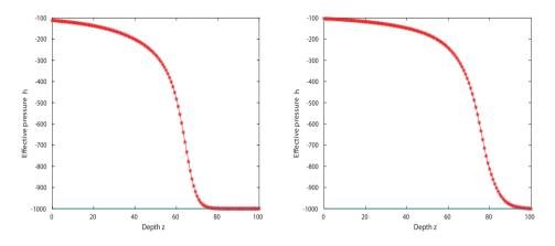
Figure 3: Head water in 14 days (left) and in 19 days (right)
