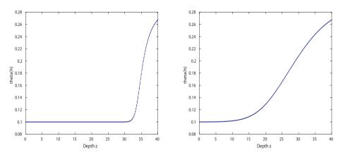
Figure 11: Water content in 5 days (left) and in 25 days (right)
